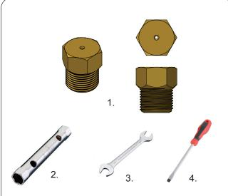
Required parts/tools: nozzles (1), box spanner 7 mm (2) open-ended spanner 7 mm (3), flat-blade screwdriver (4).
