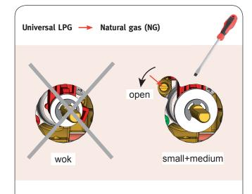
Turn the burner valve adjustment screw 1/4 anti-clockwise (open).
