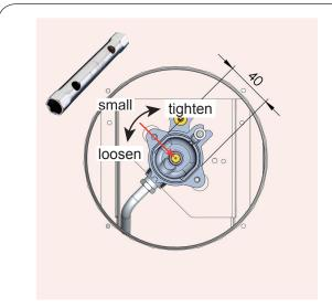
Replace nozzle small burner. Loosen the existing nozzle (anti-clockwise). Tighten the new nozzle (clockwise).
