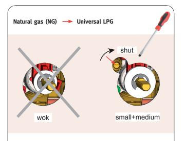
Turn the burner valve adjustment screw clockwise fully shut.
