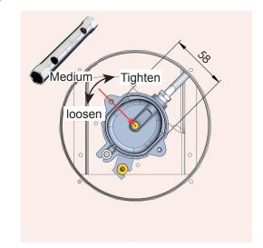
Replace nozzle medium burner. Loosen the existing nozzle (anti-clockwise). Tighten the new nozzle (clockwise).
