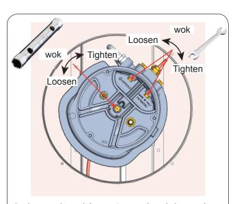
Replace nozzles wok burner. Loosen the existing nozzle (anti-clockwise). Tighten the new nozzle (clockwise).
